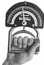
Hand dynamometer: used for testing hand grip strength.
